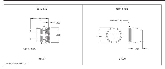
The Chicago Miniature Lamp Gemlite Indicator Light is a versatile design capable of accepting all T-1 sub-midget flange based lamps. These high quality indicators provide reliable service in a vast array of military and commercial applications where a miniature relampable front panel indicator is required. The lamp is not included with this indicator light. Please order the required lamp separately.
